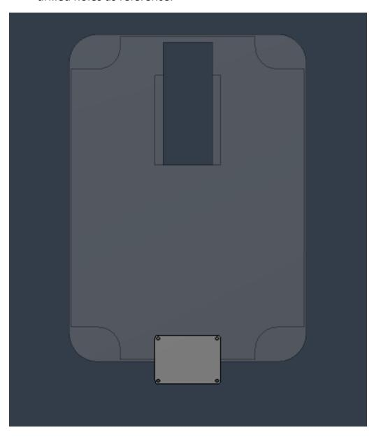
g. Install the 60% Delete top. Once in place and alignment is achieved, tighten all bolts down to a nice hand tight snug fit. DO NOT OVERTIGHTEN.
