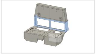
9. Install the upper seat belt bolts through the slots in the Upper Decker. Install the MOLLE panel in the Upper Decker.
