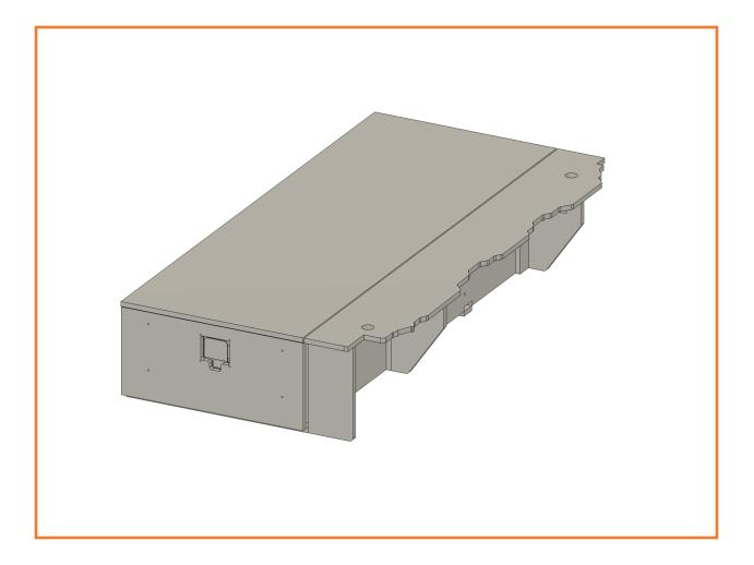
1. Begin by installing the wing cap and wing. Make sure the wing and wing cap are oriented in the correct direction when installing them into the threaded holes in the drawer system. There will be extra holes in the side of the drawer system, use the holes that line up with the hinges on the wing when the wing is lined up with the top of the drawer system.
