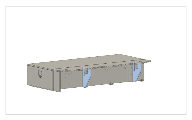
4. Check to make sure the middle L Brackets are installed on the drawer system. Install them with the included screws if they aren't already installed. Yours may be slotted. Line them up with the threaded inserts already installed in the side of the system.
