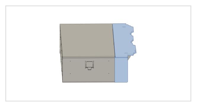
2. The wings can be adjusted to pull them closer to the drawer system and to level them with the deck of the drawer system. Just make sure the the wing has a big enough gap between it and the drawer system that it doesn't rub on the corner where the wing hinges up. The top screw adjusts the horizontal plane and the bottom screw adjusts the vertical plane of the wing when in the down position. Use a screw driver to make your adjustments.
