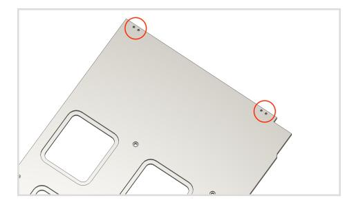
5. Place the back wall into position. Using the holes as a guide, mark the spots to be drilled in the rear window cover panel. MAKE SURE THE WINDOW IS ALL THE WAY UP. First cut through the factory insulation panel, then replace the back wall and mark the panel to be drilled. You may find it easier to remove the MOLLE panel while marking.
