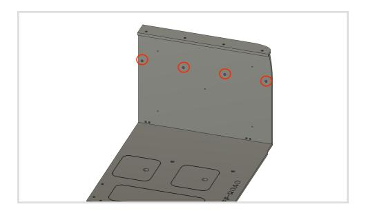
6. Remove the rear window cover panel and drill the holes at the marks made in step 5.
