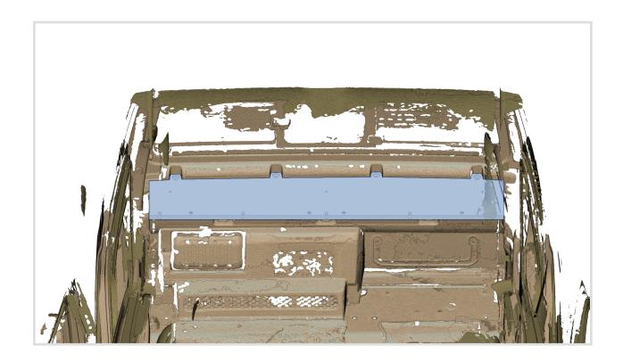
4. Install the Upper Decker Cabinet using the bolts removed from the cabinet in step 2. Do not install the seat belt bolts through the side slots yet.
