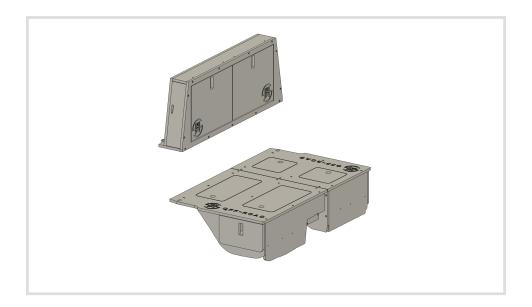
6. Screw the mid panel filler plates to the mid panel using the square head screws. Install the mid panel between the Upper Decker and Seat Deletes. Line up the holes with the cross dowels and install the bolts from the bottom and top of the mid panel, through the seat deletes and Upper Decker respectively. You may need to force the upper decker up slightly to fit the mid panel in place.
