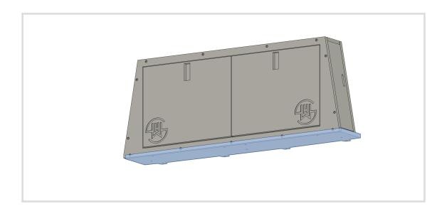
3. Install the Upper Decker Base Plate using the factory hard top bolts.
