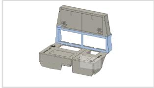
7. Install the upper seat belt bolts through the slots in the Upper Decker. Install the MOLLE panel in the Upper Decker.
