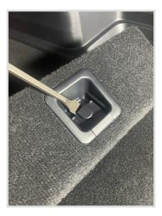
3. Remove the trim piece behind the rear seats. Install the included L brackets using the factory tie down bolts.
