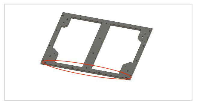
2. Grab the driver side panel and load the dowel holes with threaded dowels (the dowel holes are the end of the keyholes). Use a screw driver to line the threads up with the keyhole, the flathead slot should be facing out to make it accessible.
