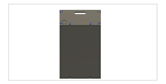
13. Repeat steps 9-12 with the second drawer. Test fit the drawers in the chassis. If they are too tight then grab a soft mallet and tap the drawer bottom in. When tapping make sure to hit the drawer bottom where the dowels are installed. Tap evenly and softly. This will make the drawer shallower and should loosen the drawer up in the chassis. Do not hit the drawer bottom too far!
