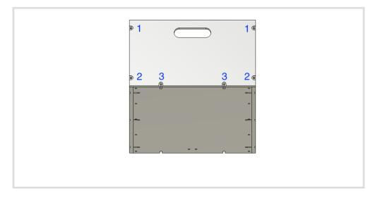
12. Flip the drawer over and do the same with the drawer front. Make sure all joints are lined up well.
