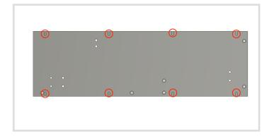
3. Attach the driver side panel to the drawer system bottom using the black 1/4-20 screws and a 5/32" Allen key. The silver dowels face the inside of the drawer system and the two countersunk holes are located at the front of the drawer system.
