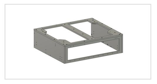
6. Attach the center divider after loading it with dowels. Note: the center divider only fits in one direction. If you find the holes do not line up then rotate/flip the piece until they do.
