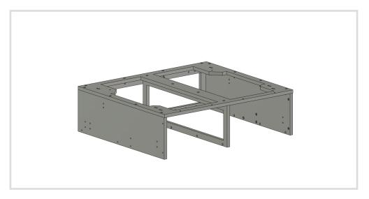
7. Flip the piece over and attach the top. Center the center divider by tapping it with a mallet.
