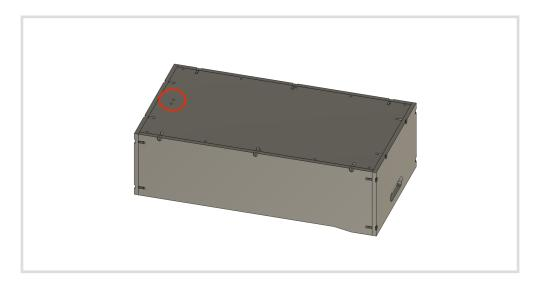
15. Place the drawer system chassis into the vehicle.
