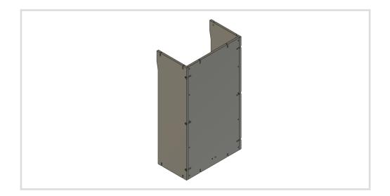
11. Load the drawer sides with dowels and attach the drawer back. Start with the top corners, then bottom corners. Finish off with the bottom two.
