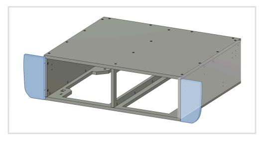
17. Attach the wing supports from the inside of the chassis at the rear. The dowels face down.
