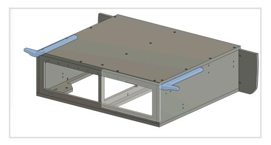
18. Install the drawers into the drawer chassis. Anchor the drawer system to the vehicle.
