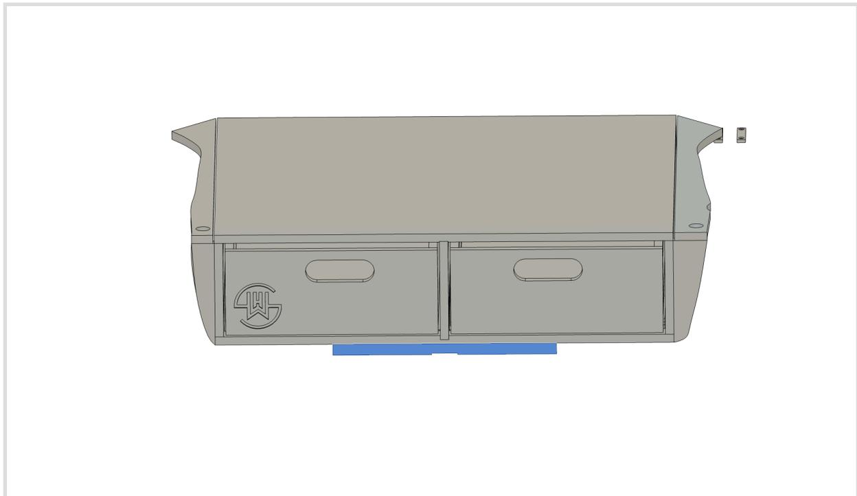
4. Slide the drawer system into the vehicle. Be careful with the wing cap on the driver side. Make sure the wings are in the upright position when you go to slide the system into the cargo area. Check to make sure the support bar is resting on the lip of the spare tire area and that the front edge of the drawer system looks level. Small shims may be required to get the drawer system level with weight in and on it. Install the passenger side wing cap.
