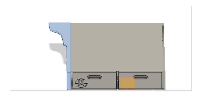
5. Shuffle the box so that you have the clearance to install the wing and the wing cap. The screws are driven from the inside of the chassis, find the predrilled holes. Start all the screws then drive them through once the pieces are lined up. Do not over tighten the screws! Install the wing cap before the wing. This step will require some patience, take your time.
