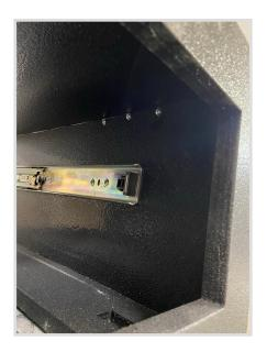
6. Line up the system and check to make sure you are happy with all the gaps with the trim. Install the mounting bolts in the base of the system. One in each corner will suffice. They only need to be snug, do not over tighten! Use hand tools for this step.
