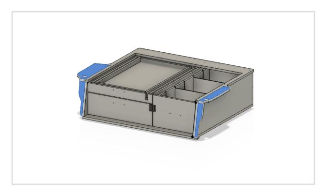
Optional: Install the wing caps before sliding the system in the vehicle. You must be careful not to slide the system in too far and brake off the wing caps, but the wing caps are easier to install this way. Use a 3" long T10 bit to install the wing cap screws. The driver side wing cap screws are driven at an angle. You will need to open the driver side drawer and fridge tray to gain access to the holes. Please contact us if assistance is needed, take your time.
