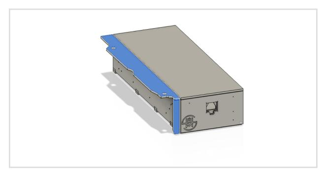
2. The wings can be adjusted to pull them closer to the drawer system and to level them with the deck of the drawer system. Just make sure the the wing has a big enough gap between it and the drawer system that it doesn't rub on the corner where the wing hinges up. The top screw adjusts the horizontal plane and the bottom screw adjusts the vertical plane of the wing when in the down position. Use a screw driver to make your adjustments.
