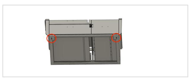
7. Loosely install the OEM tie down bolts through the base of the drawer system.
