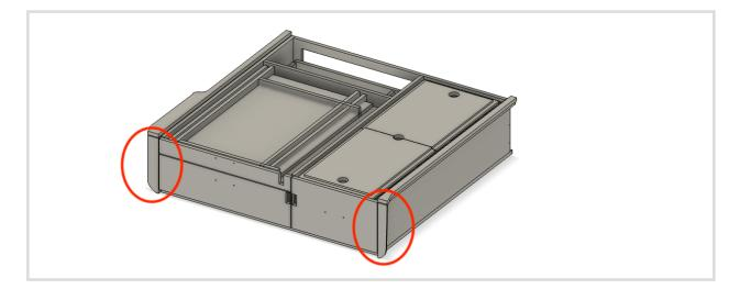
9. Install the wings of the systems using the existing holes and the included screws. The screws should be installed from the inside.
