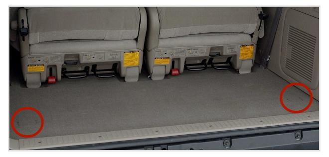
3. Layout the included blue tie down straps so that they loop through the third row anchors. Make sure to leave enough strap that the cam lock end is positioned where the second row seats fold down (it is easiest to have your second row folded up). There will not be much room on the sides when the system is in the truck.
