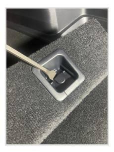
3. Remove the trim piece behind the rear seats. Reinstall the factory tie downs with the original hardware.
