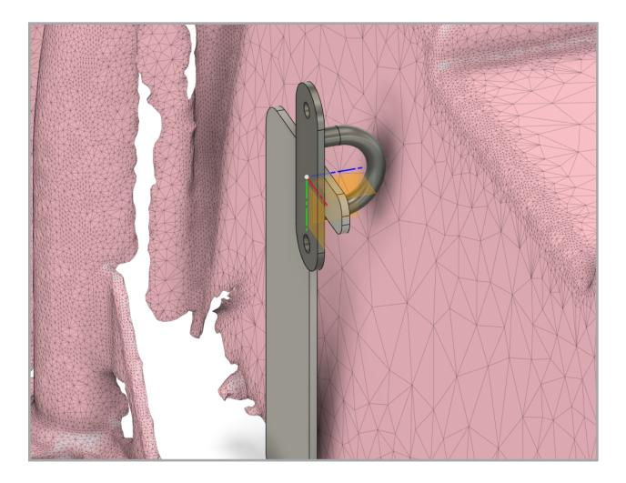
8. Use the included turnbuckles to attach the tailgate side D-ring to the bracket that was installed on step 3/4.
